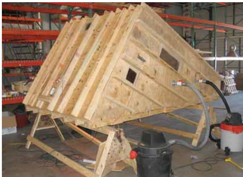
Wind load test Chamber ASTM E-330
