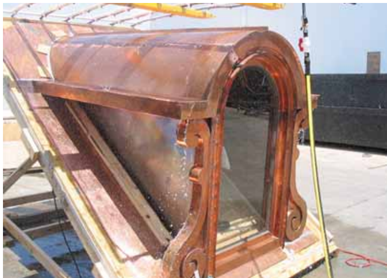
Water penetration test ASTM E-331
