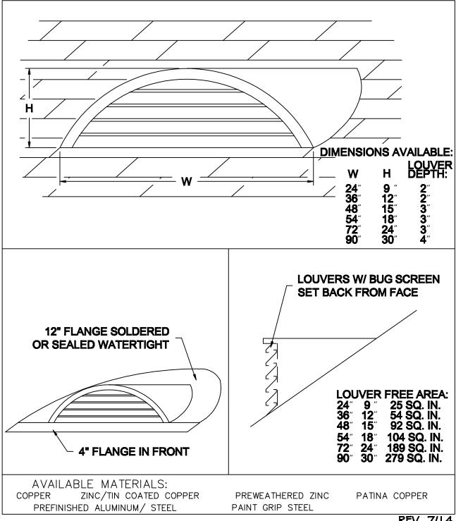
MARK OPENING IN ROOF DECK ON DESIRED COURSE. CUT OPENING IN DECK. POSITION DORMER OVER OPENING AND FASTEN TO DECK. **INSTALLATION:**
